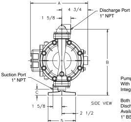
Pump Shown With 530-028-550 Integral Muffler
