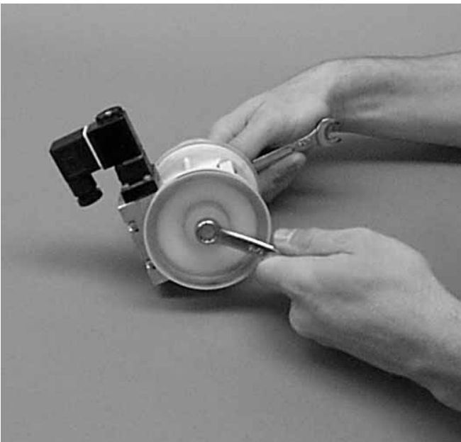
Step 10. Figure 10 Remove outer piston with \frac{1}{8} " wrench if Rubber/TPE fitted pump. For Teflon® diaphragms, remove diaphragm by turning in a counter-clockwise direction. (Figure 10)
