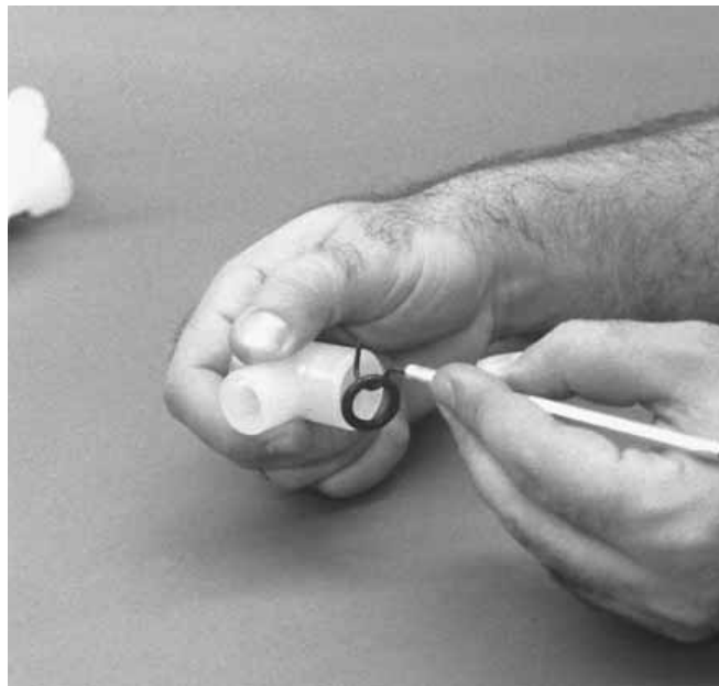
Step 9. Figure 9 Carefully remove tee-section O-ring. Inspect O-ring for wear and replace with genuine Wilden parts if necessary. (Figure 9)
