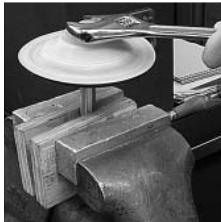
Step 12. Figure 12 To remove the remaining diaphragm assembly from the shaft, secure shaft with soft jaws (a vise fitted with plywood or other suitable material) to ensure shaft is not nicked, scratched, or gouged. Using an adjustable wrench, remove diaphragm assembly from shaft. Inspect all parts for wear and replace with genuine Wilden parts if necessary. (Figure 12)
