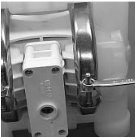
Step 7. Figure 7 With a 1/2" box wrench, loosen the large clamp bands that secure the liquid chambers to the center section. (Figure 7)
