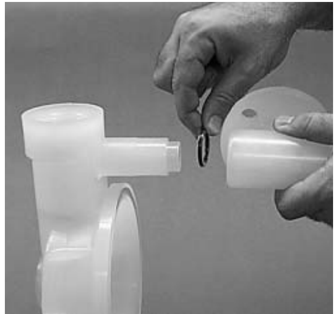
Step 10. Figure 10 Remove tee section from liquid chamber and inspect O-rings for signs of wear. Replace worn parts with genuine Wilden parts for reliable performance. (Figure 10)
