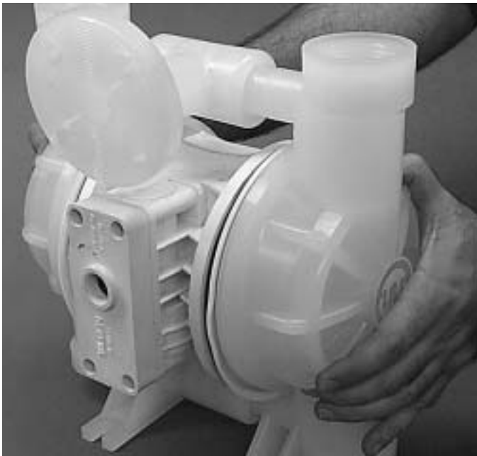
Step 9. Figure 9 After clamp bands are removed, pull liquid chambers apart. (Figure 9)
