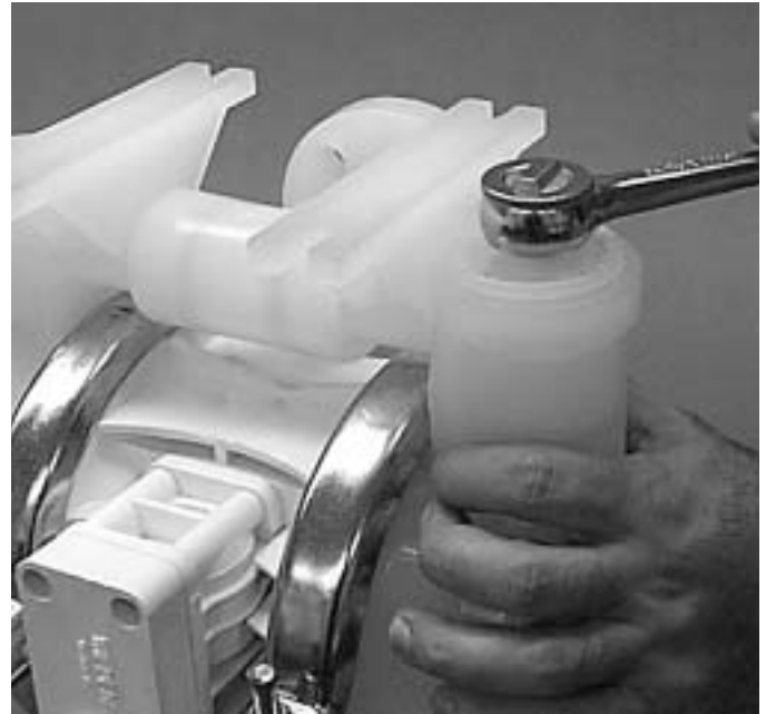
Step 5. Figure 5 Using a 1/2" socket driver, loosen the bottom retainers. (Figure 5)
