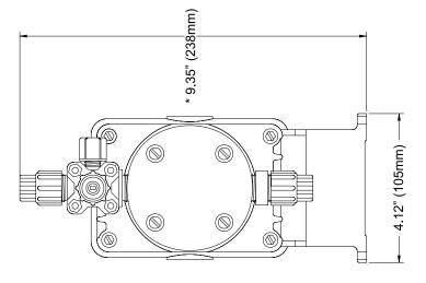
\* Dimensions shown are maximum for largest liquid end available. These dimensions vary depending on the Liquid End selected.
