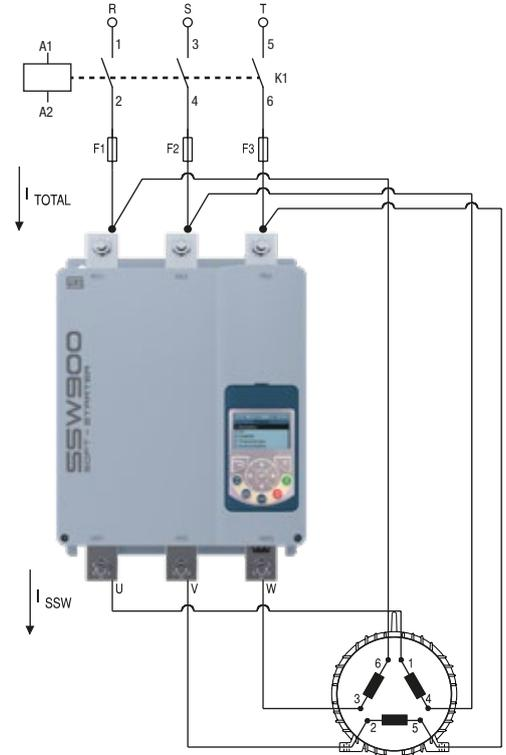
$$I_{\text{Arranc. Suave}} = \frac{I_{\text{Total consumida}}}{\sqrt{3}} = 58\% \text{ da } I_{\text{Total consumida}} \text{ (Luego del arranque)}$$
